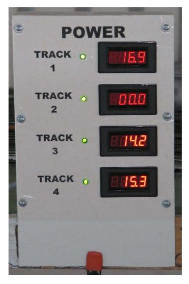
I added a power monitor to the layout. This monitor can be mounted on the powered corner and is connected to the main power box using a removable cable.
