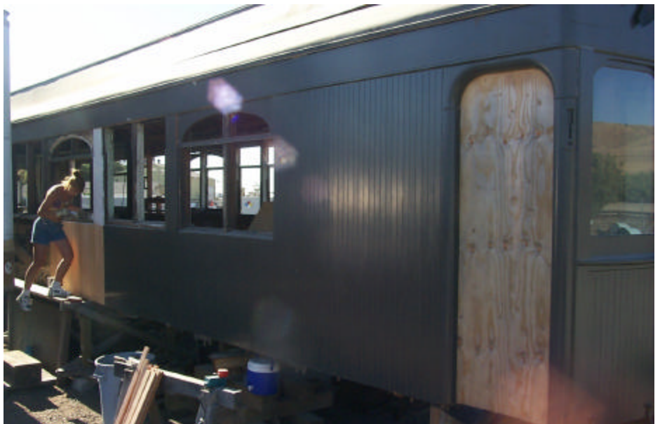
Claudia Swift priming the new siding on the right side of the car - 2002 Photo by Wes Swift
