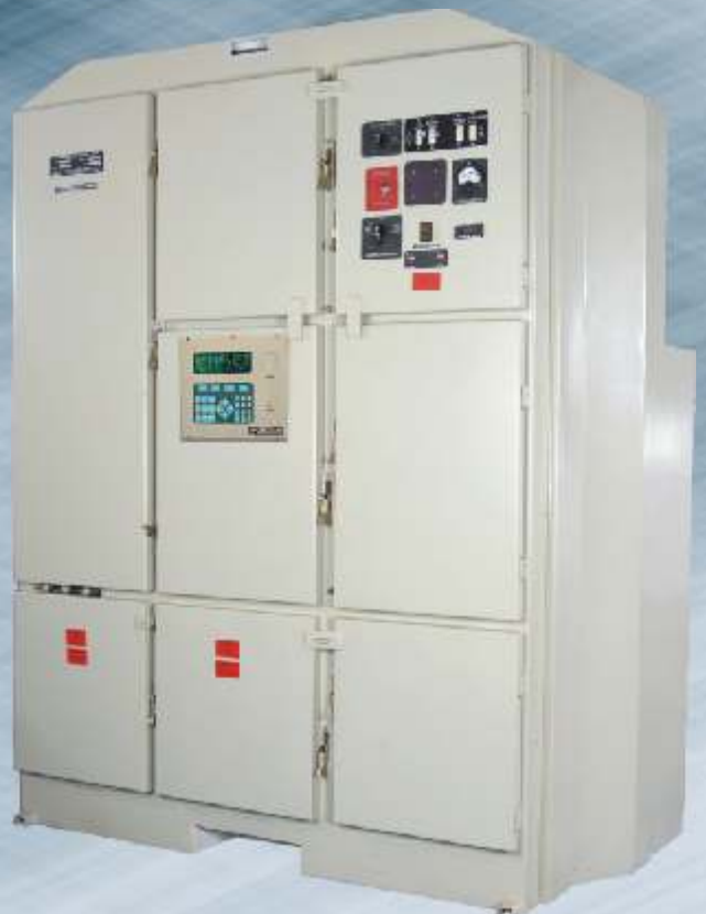
ELECTRICAL CONTROL CUBICLE WITH LOCOMOTIVE CONTROL COMPUTER
