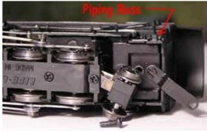
□ Lift boiler and cab straight up from frame and drive train. Note location of loose weight in boiler shell.
