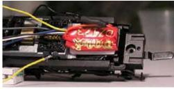
Using a small screwdriver, carefully and gently pry up the top brush holder just enough to free the clip underneath it. Exercise caution so the brush holder is not completely removed (freeing the motor brush and spring assembly). This clip has two (2) black and one (1) red wires soldered to it and also wraps around the front of the motor with a small tab that fits into the end of the motor.
