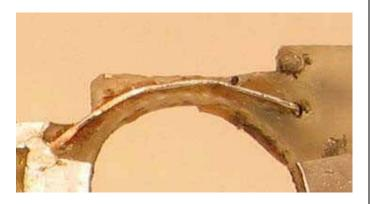
□ Flip the circuit board over, and clip off the extra wire, leaving a short length (at least 1/8") to solder the decoder to. Tin this short end of the wire. (See picture below.) This extends the power pickup trace to a place where we can solder the decoder lead directly to it.
