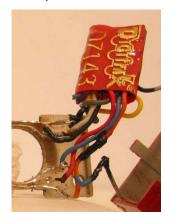
Note the special blue wire trimming for directional light requirements. It is much easier to solder the leads closest to the decoder first, and work your way across the circuit board away from the decoder. Carefully fold the decoder back over the wires onto the top of the circuit board. To insulate the leads from the body, use liquid electrical tape at all points where the new wires might contact the body or each other. Note: this insulation is not shown in the photograph below.
