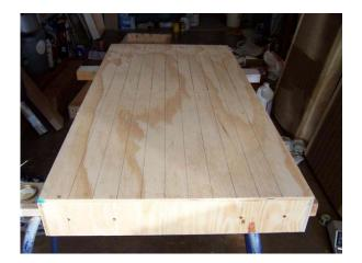
Assembled module less track and scenery. Note: the standard drill holes. Holes are required to be in exact position on all modules for the purpose of mounting modules together. The plywood top is 1200mm x 600mm x 6mm
