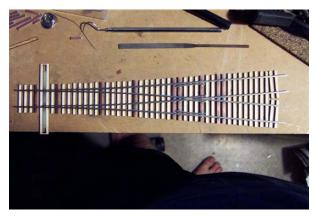
All turnouts with the exception of the yard are supplied at cost to members by MWMR. Due to the decision to use Peco Code 83 rail, and most turnout styles not being commercially available by Peco the MWMR group decided to make their own turnouts, wyes and double crossovers. The result is far superior, smoother track as demonstrated in the picture.
