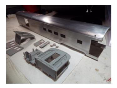
Starting in mid September, the car was gutted and the aluminum body shell stripped using a strong paint remover. ( Don't use this stuff on plastic body shells!)
