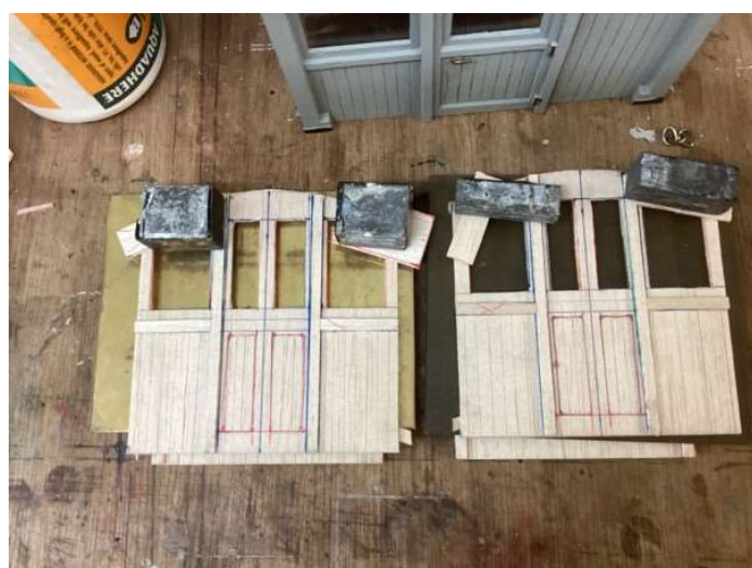
Plywood fretted, curved roof ribs glued to end walls.
