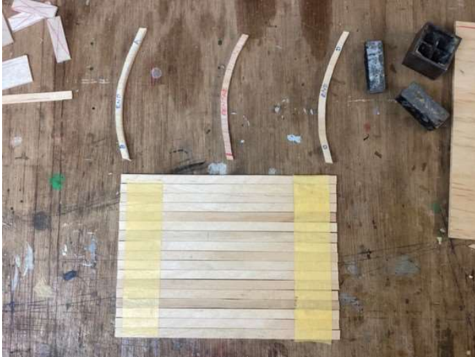
Roofing slats, squared up and taped from inside.
