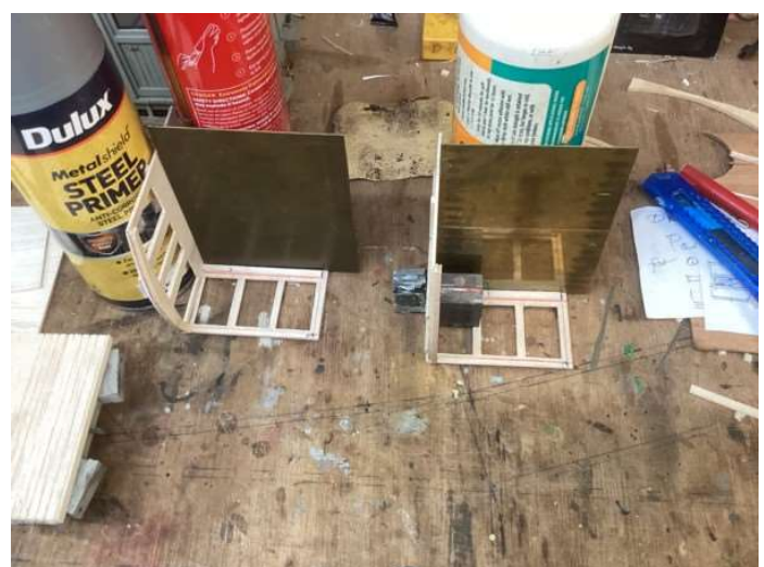
End walls and side walls held square while glue sets.
