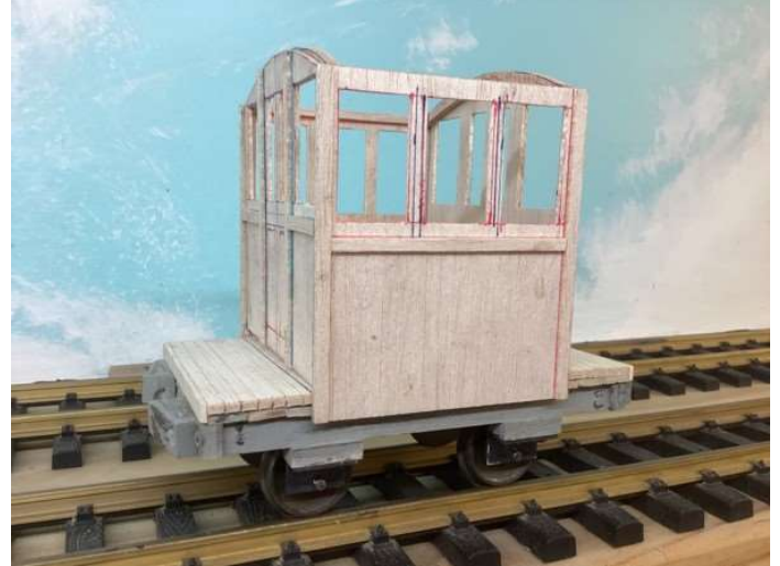
Body shell ready for glueing roof slats overlay.
