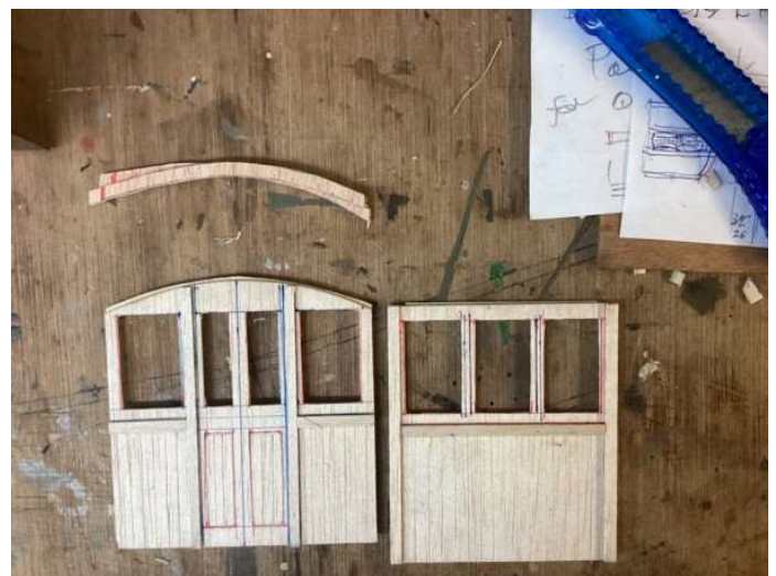
The bottom edge of side walls fit over the ends of floor planks to retain the body from moving laterally.
