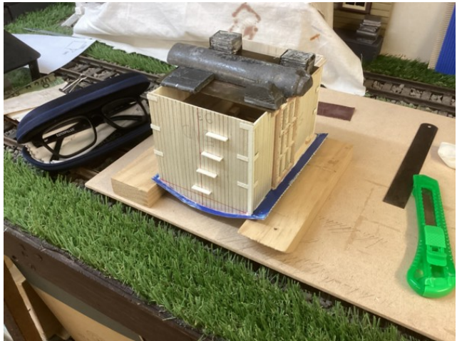
Corrugated Galvanized roofing is trimmed and then glued to ribs and stiffeners, weight added to press on.
