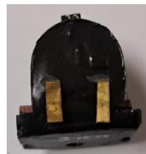
These are inserted right behind the brush cap and can drive the lights without additional wiring. The resin cast inserts also can accommodate Artista figures of engineer and fireman.
