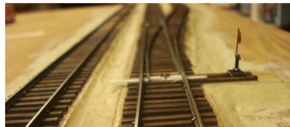
This is a manual operating switch stand
