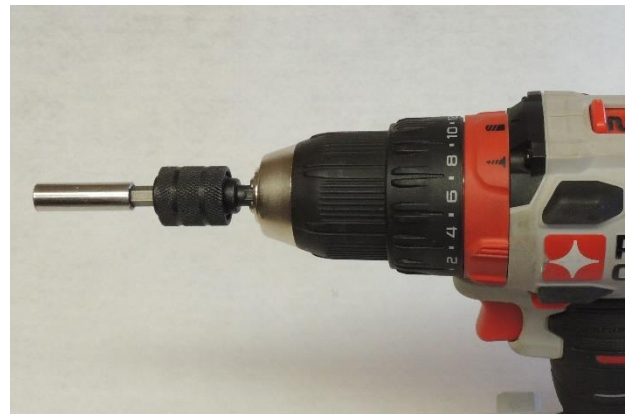
A drill with 1/4 inch hex driver: a very quick way of swapping 1/4 inch hex bits.
