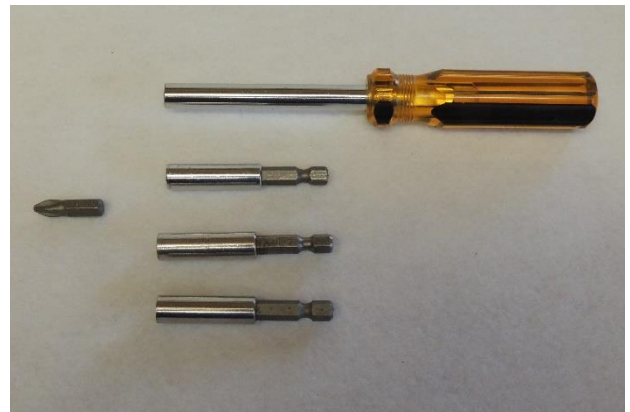
Set of 1/4 inch hex driver and extensions: used when there is not enough room for a regular screw driver.
