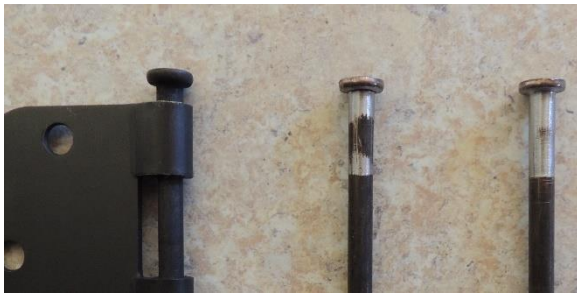
Left to right, Stock pin, thick shoulder ground down, pin diameter further reduced.
