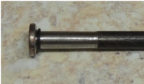
O-ring added to make pin removal easier."
