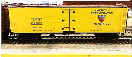
This car is from the first set of "kits" (24000-24099) supplied by A.C.&F. to A.R.T., to be built in their St. Louis shops. 1931 – 1947 Paint Scheme shown. Intermountain HO Scale // Note: Horizontal Seam (only model like prototype)
