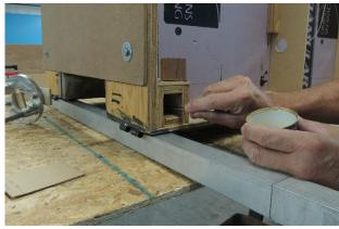
To reinforce the leg pockets, glue is first applied to the inside of each pocket in the bottom inch.
