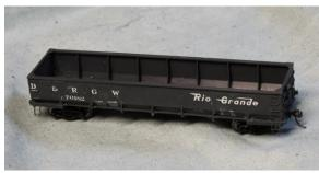
He noted that "GS Class gondolas were extensively used by western railroads instead of hopper cars because of their flexibility: they could be used for a variety of different loads. This gondola was a 46-foot, 70-ton that was probably the largest ever built and was exclusively built for the Rio Grande, which eventually owned about 700 cars. They were built from the 1920s
