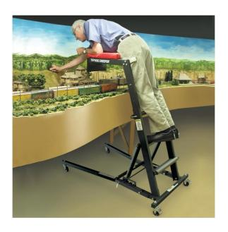
A topside creeper is a step ladder to which a shelf has been added allowing the model railroader to reach into the layout.
