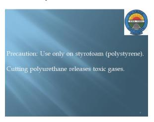
and lastly, a warning to cut only styrofoam with a hotwire cutter.
