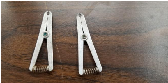
Aluminum, spring loaded heat sinks.
