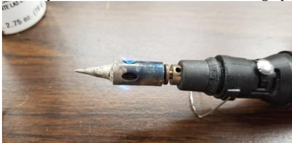
Solder pen now hot (internal heating mesh is red)
