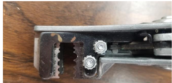
Wire strippers, note wire gauge sizes, 10 to 22 gauge.
