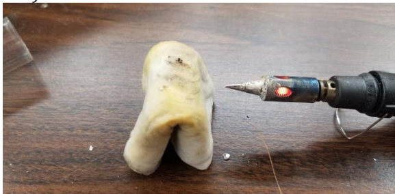
Clean tip and wipe on wet paper towel or sponge. If using sponge, don't press down hard, sponge will launch solder at you.
