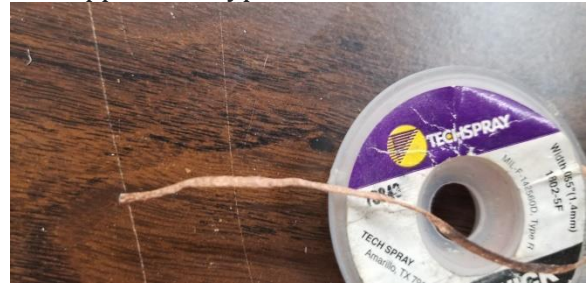
Copper braid. Used to remove solder from a connection.
