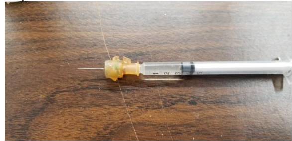
Flux applicator, hypodermic needle.
