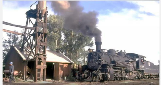
What good is coal if we don't have sand to get started? Sanding tower for narrow gauge.
