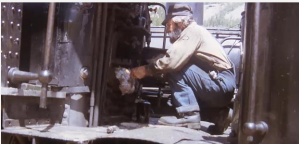
Starting up a cold boiler requires a bunch of oily rags and a signal flare.
