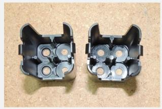
There are two styles of battery holders. Flat top and button top and my new batteries are button top. The left battery holder is designed for the button top and the right is designed for the flat top batteries. Place four batteries to the one on the left. The button top (+) goes in the left side.
