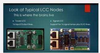
The signal-LCC can control and drive 16 LEDs.
