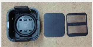
First, an O-ring is placed in the bottom. Next a spacer is made to fit and then two brass strips are made to connect the two sets of batteries. Glue the strips to the spacer.
