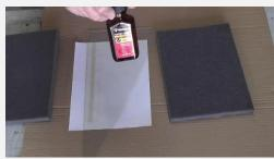
**One:** Glass is used as a carrier for contact cement to glue two pieces of foam together. The area of the glass is coated with contact cement to cover the section of foam needed to glue the pieces together.
