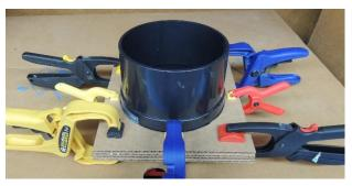
I then made an adapter plate out of four layers of cardboard with a 4" hole cut out. Next I glued the cardboard to a 4"pipe hose adapter (Home Depot SKU # 1001839325). I use gorilla glue as it expands when it dries.
