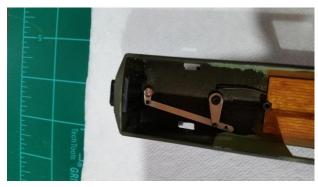
I carefully cut away the melted top of the coupler shaft, cleaned up the top, making sure to leave the rectangular top of the shaft flush with the fulcrum. I removed the coupler box from the bottom of the car, cleaned up and smoothed all surfaces. I drilled a #66 hole and inserted a self-tapping screw/washer to hold the coupler box in place and to lock the fulcrum. The mechanism worked as good as new!
