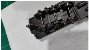
After successfully shimming and replacing couplers in several other cars, I managed to touch up too much CA to some shims and accidentally glued one coupler pocket to the car. After a lot of prying I was able to 'break' the CA grip, and after a lot of digging, I removed most of the CA residue. Unfortunately, the coupler pocket would not move smoothly and caused the truck not to rotate freely. I was forced to remove the rotating coupler box to make things work better.
