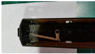
Upon removal of the single piece roof+clear window shell, I found that the coupler box had a shaft extended into the car body, which was 'melted' down on top of the fulcrum attached to the truck.
