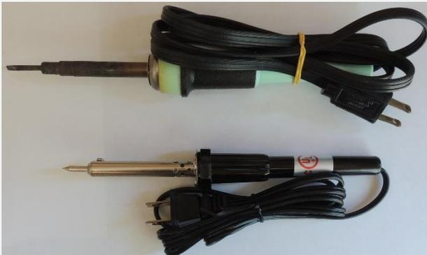
Various manufacturers have made pointed tip soldering irons (bottom of photo above) that are held in with a set screw. My opinion of these soldering irons are that they are prone to poor heat transfer. Enter the 21<sup>st</sup> Century. With its slowly shrinking electronics, these irons are not the best for microelectronics.
