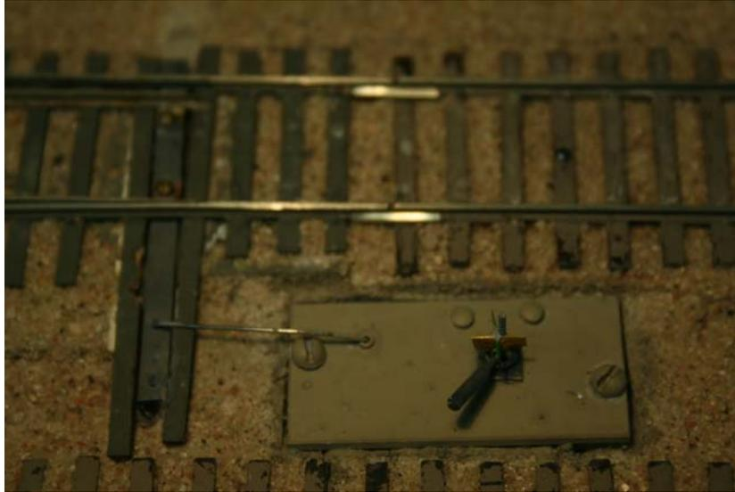
Figure 9: Installed Low Ground Throw
