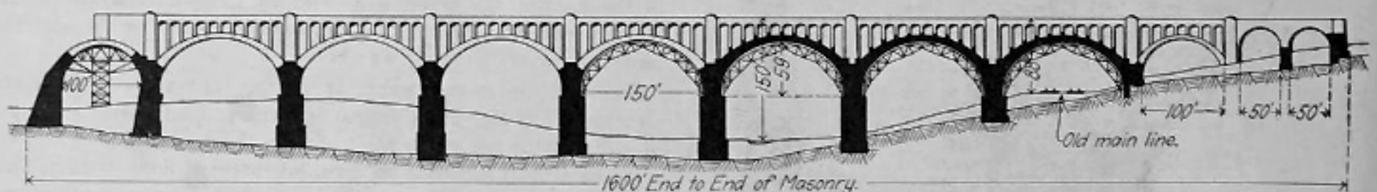
Elevation of Martin's Creek Viaduct, Showing Progress to November 1.
