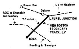
The New Boston Secondary Track extends from Laurel Junction (Milepost 157.5) to Rock, Pa. (Milepost 167.1), a distance of 9.6 miles, in Schuylkill County, Pa. At Laurel Junction, this line connects with the Lehigh Valley line to Hazleton and the Lehigh Valley Delano Secondary Track to Kohinoor Junction. A portion of the latter line is also under study in this Report.
